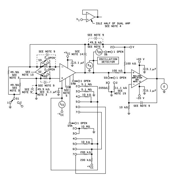
FIGURE 3. Test circuit for static and dynamic tests.
