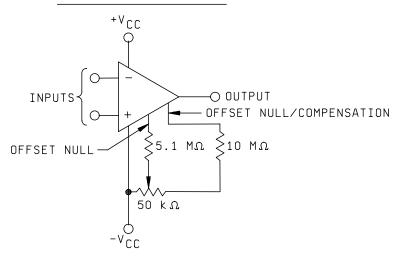
FIGURE 2. Offset null circuits.
